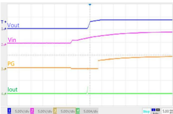
V IN 开机 V_{OUT}=3.3V , I_{OUT}=0A
