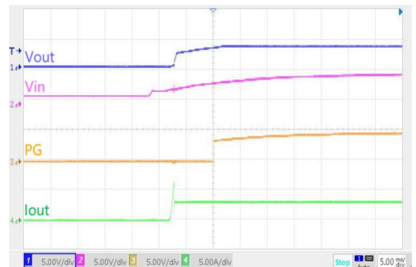
V IN 开机 V_{OUT}=3.3V , I_{OUT}=3A
