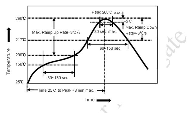
\*Above reflow soldering curve is from J-STD-020D.
